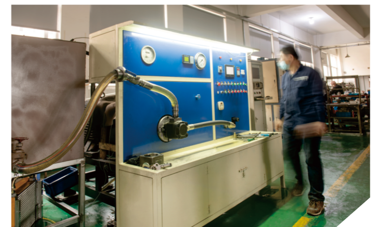
内啮合泵测试台 Internal Gear Pump Testing Equipment
