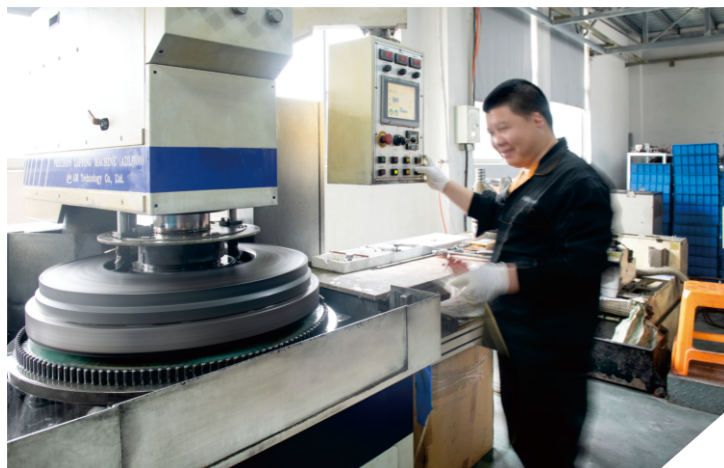
双端面磨床 Paralled Surface Grinding Machine
