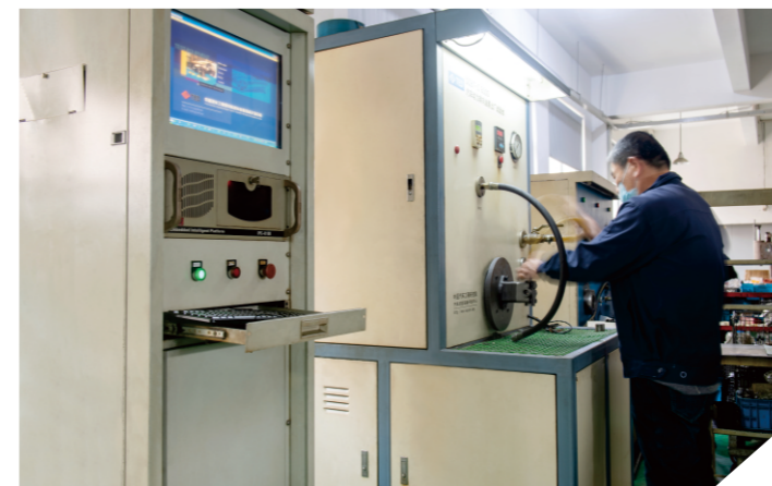
叶片泵测试台 Vane Pump Testing Equipment
